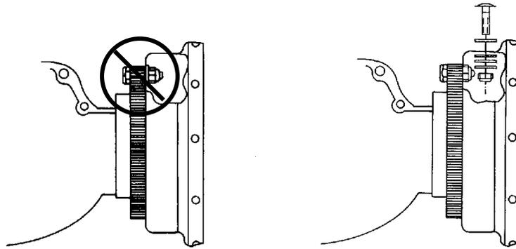
On any engine that has the spinner bulkhead attached directly to the starter ring gear, do not attach weights to the bolts that retain the spinner bulkhead to the starter ring gear. This installation requires that the weights be installed on the inner portion of the spinner bulkhead.
