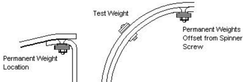
Install weights on the spinner bulkhead by installing a counter sunk screw into the flange. The hole should be offset from the spinner screw approximately four times the diameter of the installed screw. Holes must be drilled undersized and reamed to final dimension.
