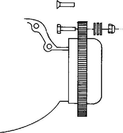
Weights can be attached to some starter ring gears. A bolt and weight may be installed if the ring gear has equally spaced, unoccupied holes.
