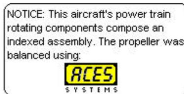
Example of placard to be placed on propeller assembly.
