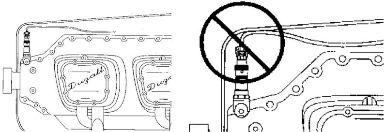
Mount the vibration sensor vertically, close to the engine centerline, with the cable pointing up. If you can't attach the vibration sensor exactly on the engine centerline, you can still get accurate results by attaching the sensor to the front bearing retaining bolts.
