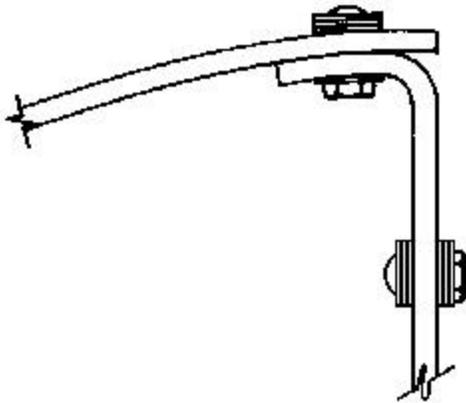
Install weights on the backing plate by drilling the backing plate and bolting equal amounts of washers on both sides of the bulkhead. Holes must be drilled undersized and reamed to final dimension. The amount of weight installed must be increased to account for the difference in radius of the test weight and the permanent weight radius.
