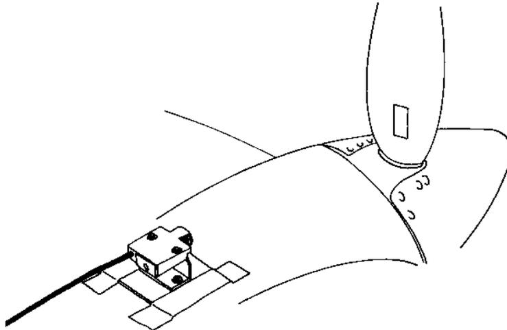
Route the vibration sensor cable and the photo tach cable to the cockpit, keeping the cables away from moving parts of the engine, hot manifolds, and hot oil lines.
