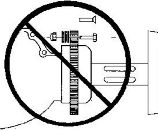
Lycoming installations that use a long spacer between the ring gear and the propeller may not respond correctly to weights applied to the ring gear. These installations require that the balance weights be attached on the spinner bulkhead.
