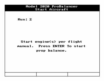
The "Start Aircraft" banner screen indicates the upcoming run number and directs you to "Start engine(s) per flight manual". Press [ENTER] to start prop balance." Then repeat the procedures described above starting with item, 4.1.6 until the level of vibration is at or better than an acceptable level. See the *ACES Systems Guide to Propeller Balancing* for details of vibration levels and weight installation procedures.
