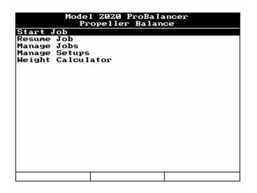
Selecting "Start Job" from the "Propeller Balance" banner screen allows you to begin a new propeller balance job. When you select this option, one of three screens will appear depending on whether you are: 1) Starting a new job with no setups previously defined in the analyzer's memory; 2) Starting a new job with previously defined setups available in the analyzer's memory; or 3) Resuming an incomplete job being held in the analyzer's memory.
