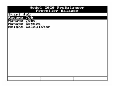
Selecting "Resume Job" from the "Propeller Balance" banner screen menu allows you to select a job to resume. Using the  $[\downarrow]$  key, highlight the job you wish to complete from the list of incomplete jobs, and press [ENTER]. You will be taken to the last step completed in the job process.
