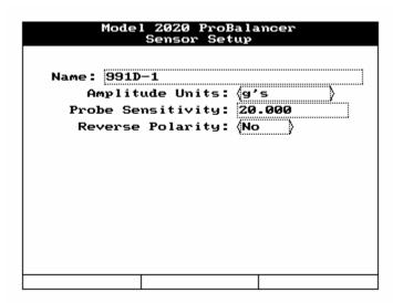
This is an information-only screen for use in verifying the parameters of the vibration sensor you have chosen. You may not edit or otherwise enter information on this screen. If this sensor does not possess the specifications you require for this setup, you may enter a new sensor in the "Sensor Setup" screen, or choose another sensor from the existing list. Press [BACKUP] or [ENTER] to exit this screen and return to the "Prop Balance Setup" banner screen.
