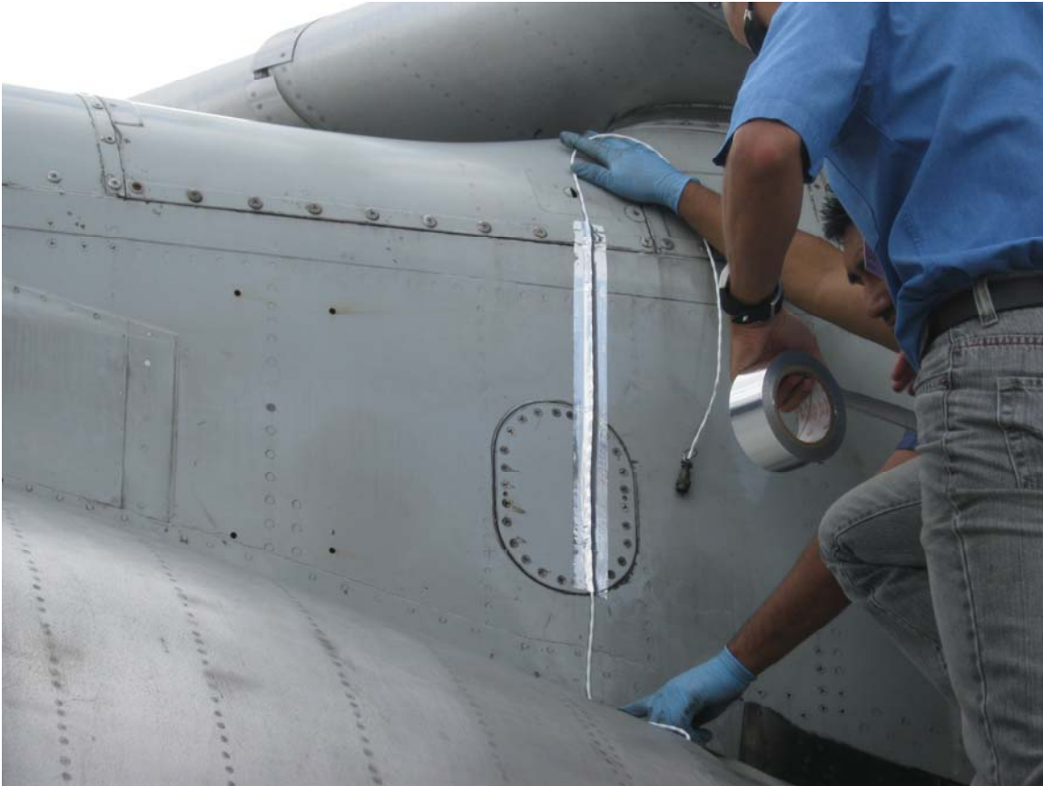
Figure 5. High Temp cable routed from the vent, up the pylon and to the top of the wing. Speed tape must be used in the bypass air stream to insure security of the cable.
